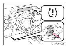
5 Vehicles without a smart key system: Wait for a few minutes with the engine switch in the "ON" position and then turn the engine switch to the "ACC" or "LOCK" position.
