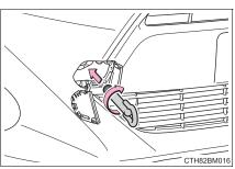
5 Tighten down the towing eyelet securely using a wheel nut wrench or hard metal bar.
