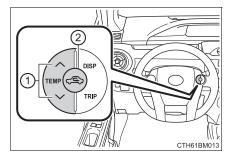
The mode switches between outside air mode and recirculated air mode each time  $\$  is pressed.
