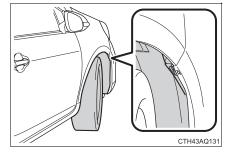
2 Partly remove the fender liner.
