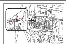
4 Check if the fuse is blown.▶ Type A
