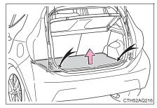
2 Remove the jack after removing the hook.
