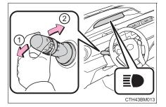
You can flash the high beams with the headlights on or off.
