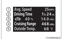
EV driving rate and driven distance (percentage and distance driven using just the electric motor [traction motor] only) will be displayed.
