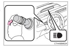
2 Press the Automatic High Beam switch.
