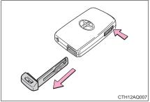
After using the mechanical key, store it in the electronic key. Carry the mechanical key together with the electronic key. If the electronic key battery is depleted or the entry function does not operate properly, you will need the mechanical key. ( $\rightarrow$ P. 516)
