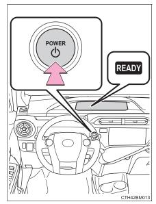
If the "READY" indicator changes from a flashing light to a solid light and a beep sound, the hybrid system is starting normally.
