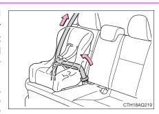
6 If the child restraint has a top tether strap, the top tether strap should be latched onto the top tether strap anchor. (→P. 69)
