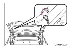
2 Pull the luggage cover backward to disengage the anchors.
