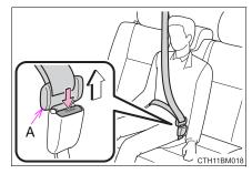
2 To release tab "B", insert the key (→P. 120) or tab "A" into the hole on the buckle.
