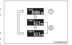
Pressing and holding the "TRIP" switch will reset the trip meter.
