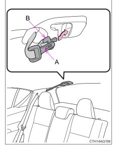
With tab "B" inserted all the way into the cover, move tab "A" slightly back toward the cover's inlet, so that it blocks the inlet.
