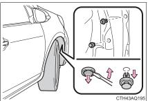
3 Partly remove the fender liner.
