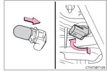
7 Connect the connector. (When replacing right side bulb only.)
