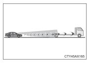
If a vehicle ahead has extremely high ground clearance
