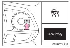
If the cruise control main switch is pressed and held for 1.5 seconds or more, the system turns on in constant speed control mode. (→P. 306)
