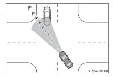
When you turn right/left, pedestrian is detected in the forward direction and estimated to enter your vehicle's path (bicyclists are detected.)
