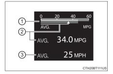
Displays the average vehicle speed since reset or elapsed time since reset, as selected in  $\bigcirc$  . ( $\rightarrow$ P. 111)
