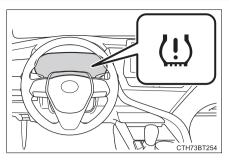
8 Vehicles with a tire inflation pressure display function: Drive at approximately 25 mph (40 km/h) or more for approximately 10 to 30 minutes.
