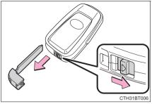
After using the mechanical key, store it in the electronic key. Carry the mechanical key together with the electronic key. If the electronic key battery is depleted or the entry function does not operate properly, you will need the mechanical key. (→P. 539)
