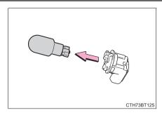
6 Install a new light bulb and then install the bulb base to the light unit by inserting it and turning it clockwise.
