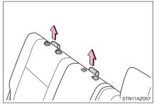
4 Route the top tether strap through the anchor strap router as shown in the illustration.
