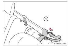
5 Latch the hook onto the anchor strap ring and tighten the top tether strap.
