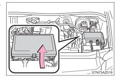
Under the instrument panel Remove the cover.
