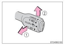
However, cruise control does not resume when the vehicle speed is approximately 25 mph (40 km/h) or less.
