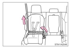
5 If the child restraint has a top tether strap, the top tether strap should be latched onto the top tether strap anchor. (→P. 70, 73)
