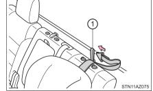
4 Latch the hook onto the anchor strap belt and tighten the top tether strap.
