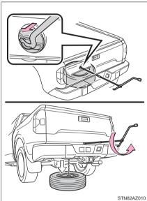
After the tire is lowered completely to the ground, remove the holding bracket.
