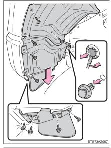
2 Open the fender liner and unplug the connector.
