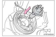
7 Install the bulb retaining spring.
