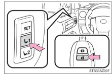
To prevent unintended triggering of the alarm, open and close a door once after a driving position has been recorded. (If a door is not opened within 60 seconds after  $\bigcap$  is pressed, the doors will be locked again and the alarm will automatically be set.) In case that the alarm is triggered, immediately stop the alarm. ( $\rightarrow$ P. 95)
