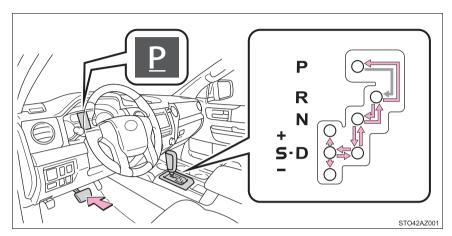
While the engine switch is in ON, move the shift lever with the brake pedal depressed.
