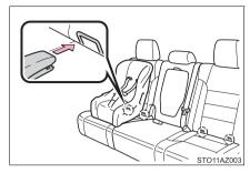
Seat belts equipped with a child restraint locking mechanism (ALR/ELR belts except driver's seat belt) (→P. 36)
