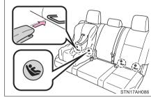
Seat belts equipped with a child restraint locking mechanism (ALR/ELR belts except driver's seat belt) (→P. 36)
