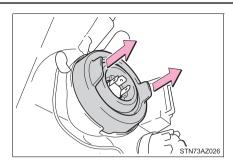
4 Release the bulb retaining spring.
