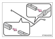
Insert the end of the jack handle extension into the lowering screw and turn it counterclockwise.
