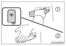
2 Touch the lock sensor (the indentation on the side of the door handle) to lock the doors.
