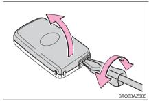
Remove the depleted battery.
