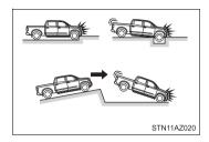
The SRS curtain shield airbags may also deploy under the situation shown in the illustration.
