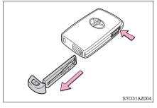
After using the mechanical key, store it in the electronic key. Carry the mechanical key together with the electronic key. If the electronic key battery is depleted or the entry function does not operate properly, you will need the mechanical key. (→P. 519)
