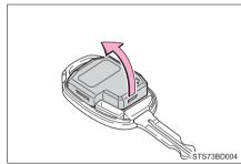
3 Open the case cover using a coin protected with tape, etc., and remove the depleted battery.
