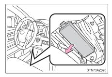
Remove the fuse with the pullout tool.
