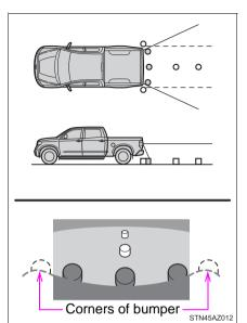
Items which are located higher than the camera may not be displayed by the monitor.
