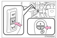
To prevent unintended triggering of the alarm, open and close a door once after a driving position has been recorded. (If a door is not opened within 60 seconds after  $\mathbf{a}$  is pressed, the doors will be locked again and the alarm will automatically be set.) In case that the alarm is triggered, immediately stop the alarm.  $(\to P. 80)$
