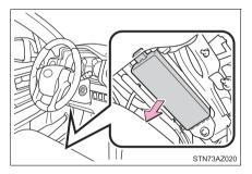
Remove the fuse with the pullout tool.
