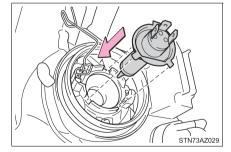
7 Install the bulb retaining spring.
