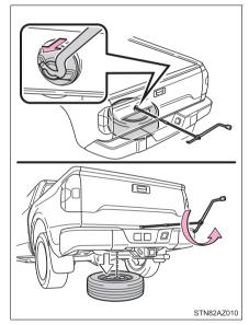
3 After the tire is lowered completely to the ground, remove the holding bracket.
