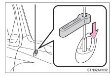
2 Loosen the antenna with the wrench and remove it.
