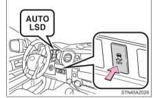
Stop the vehicle completely, and press the VSC off switch for more than 3 seconds.
