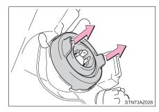
4 Release the bulb retaining spring.
