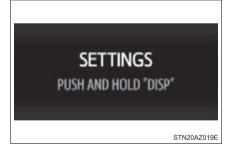
Press and hold the "DISP" button after selecting the desired setting item ("TURN BY TURN NAVI", "LANGUAGE" or "UNITS") by pressing the "DISP" button.
