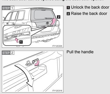
The back door can be opened using the back door opener.
