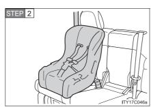
Place the convertible seat on the seat facing the front of the vehicle.
