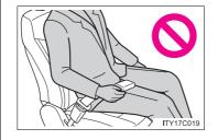
If the seat belt extender has been connected to the driver's seat belt buckle but the seat belt extender has not also been fastened to the latch plate of the driver's seat belt, the SRS driver's airbag system will judge that the driver is wearing the seat belt even though the seat belt has not been connected. In this case, the driver's airbag may not activate correctly in a collision, resulting in death or serious injury in the event of collision. Be sure to wear the seat belt extender.
