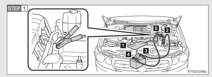
Connecting the jumper cables.
