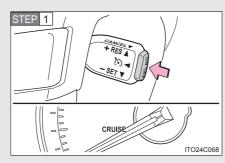
Press the "ON-OFF" switch to operate the cruise control.
