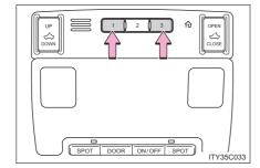
Press and hold the 2 outside buttons for 10 seconds until the indicator light flashes.
