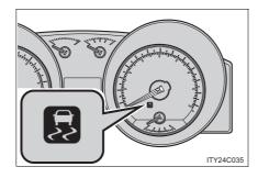
If the vehicle is in danger of slipping, rolling backwards when starting on an incline, or if the rear wheels spin, the slip indicator light flashes to indicate that the VSC/Active TRAC/hill-start assist control systems have been engaged.
