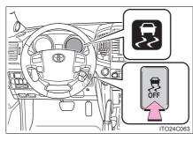
Quickly push and release the button to turn off Active TRAC.
