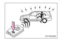
When ((()) is pressed for longer than about one second, the headlights/tail lights/emergency flashers will flash, the front and rear interior lights will come on, and an alarm will sound for about 60 seconds to deter any person from trying to break into or damage your vehicle.
