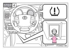
Press and hold the tire pressure warning reset switch until the tire pressure warning light blinks slowly three times and the message "TIRE PRESSURE RESET PROCEEDING" appears on the multi-information display.
