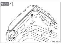
Open the back door and remove the nuts and lamp assembly.
