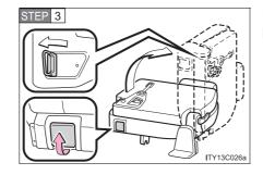
Pull the seat leg lock release levers.
