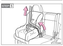
While pushing the convertible seat into the seat, allow the shoulder belt to retract until the convertible seat is securely in place.
