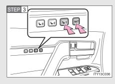
While pressing the "SET" button, press button "1", "2" or "3" until the signal beeps.
