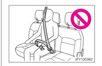
Do not use the third center seat belt with either buckle released. Fastening only one of the buckles may result in death or serious injury in case of sudden braking or a collision.
