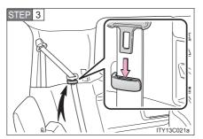
Pass the outer seat belts through the seat belt hangers and secure the seat belt plates.
