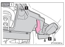
Remove the fender liner bolts, loose the fender liner nut and remove the fender liner.
