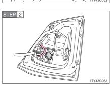
Turn the bulb bases counter-clockwise.
