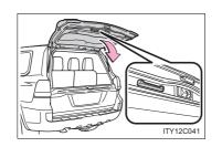
• Lower the back door using the back door handle, and make sure to push the back door down from the outside to close it.
