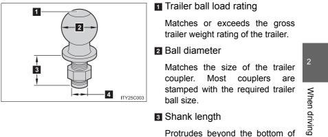
Protrudes beyond the bottom of the lock washer and nut at least 2 threads.
