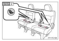
Take off the covers between the seat cushion and seatback, then confirm the position of the LATCH anchors below the symbol in the seatback.
