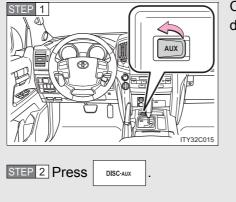
Connect the portable audio device.
