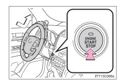
When the "ENGINE START STOP" switch is OFF, the steering wheel returns to its stowed position by moving up and away to enable easier driver entry and exit.
