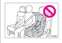
When using the left side lower anchors for the child restraint system, do not sit in the center seat. Seat belt function may be impaired, such as being positioned overly high or loose-fitting, which may result in death or serious injury in the event of a collision. Before driving
