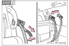
Hook the holding strap to the assist grip and secure the seat by pulling its free end.
