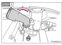
For the left side only: Remove the securing bolt and move the washer fluid filler opening.
