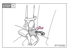
To release the hooked tab, insert the mechanical key into the hole on the buckle with the light gray buckle release button.
