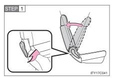
Fold the seatback while pulling the seatback angle lever. Return the seatback and secure it at the first lock position.  $(\rightarrow P. 53)$
