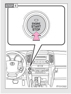
Press the "ENGINE START STOP" switch.
