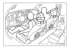
When a front seatback receives a strong impact, the head restraint moves slightly forward and upward to help reduce the risk of whiplash on the seat occupant.
