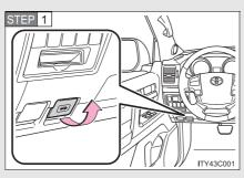
Release the lock from the inside of the vehicle to open the hood.
