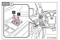
Shift the shift lever to "P" or "N", press and hold the driver's door lock switch (1 or 2) for 5 seconds then release.
