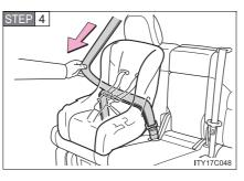
Fully extend the shoulder strap and then allow it to retract slightly into the ALR lock mode.
