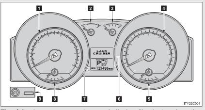
The following gauges, meters and display illuminate when the "ENGINE START STOP" switch is in IGNITION ON mode.
