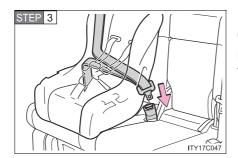
Run the seat belt through the convertible seat and insert the plate into the buckle. Make sure that the belt is not twisted.
