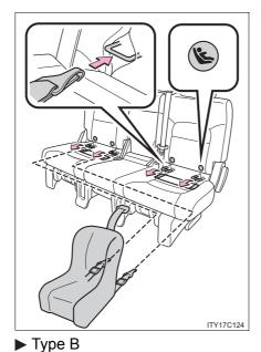
STEP 3 Latch the hooks of the lower straps onto the LATCH anchors.
