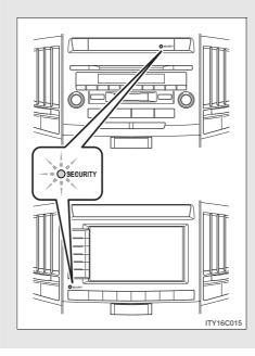
The indicator light flashes after the "ENGINE START STOP" switch has been turned OFF to indicate that the system is operating.
