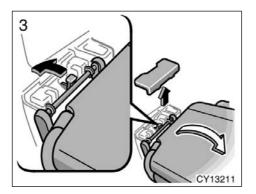
3. Remove the cover and push the seat lock release lever outward to unlock the seat lock, then pull up the whole seat and remove it. After removing the seat, reinstall the cover.
