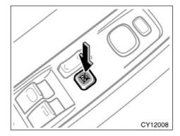
If you push in the window lock switch on the driver's door, the back window cannot be operated.
