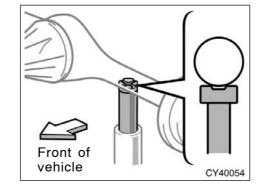
6. After making sure that no one is in the vehicle, as the jack touches the vehicle and begins to fit, double-check that it is properly positioned.
