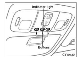
The garage door opener (**HomeLink**<sup>®</sup> Universal Transceiver) is manufactured under license from HomeLink<sup>®</sup> and can be programmed to operate garage doors, gates, entry doors, door locks, home lighting systems, and security systems, etc. (a) Programming the HomeLink<sup>®</sup>
