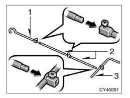
Put a jack handle, jack handle extensions and jack handle end together as shown in the illustration.
