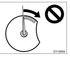
The tachometer indicates engine speed in thousands of rpm (revolutions per minute). Use it while driving to select correct shift points and to prevent engine lugging and over-revving.
