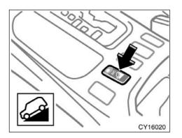
If the indicator light does not come on when the switch is pushed, contact your Toyota dealer.
