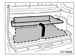
2. Hold the handle and raise the double deck on the rear tire houses.
