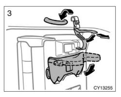
3. Stow the seat leg in the back of the seat cushion. Take the holding strap out of its holder, and attach the strap to the assist grip. Tighten the strap by pulling the end and fix it with Velcro.
