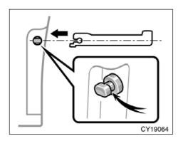
If the trash holder is pulled strongly or stepped on, it will detach from the rear console box to protect it from damaging.
