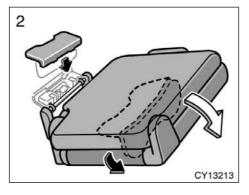
2. Pull out the seat leg from the back of the seat cushion and lock it on the anchor. Reinstall the cover.
