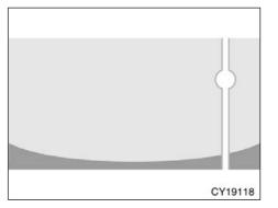
If a bright light (for example, sunlight reflected off the vehicle body) is picked up by the camera, the smear effect\* peculiar to the CCD camera may occur.
