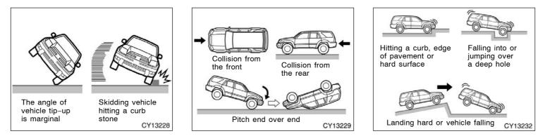
The curtain shield airbags may inflate if the angle of vehicle tip-up is marginal or if the skidding vehicle's tires hit a curb stone laterally as shown in the illustration.
