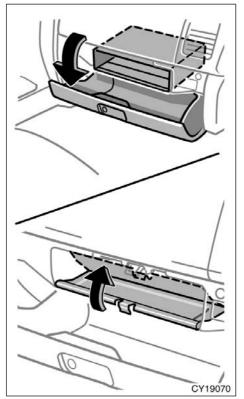
On some models, an auxiliary box is located inside the glove box.
