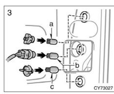
a: Rear turn signal light b: Stop/tail and rear side marker light c: Back–up light
