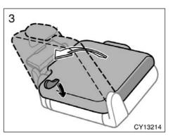
3. Raise the seatback while pushing down the seatback angle adjusting lever.
