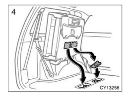
4. Remove the seat anchor covers from the back of the seat cushion, and install them over the seat anchors.
