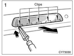
Disconnect the clips by using a flatbladed screwdriver which is wrapped with a cloth.
