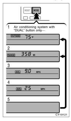
The outside temperature display (air conditioning system with "DUAL" button) and cruise information display indicates the following information.
