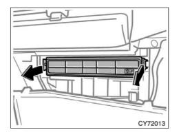
3. Remove the filter case by holding both sides.
