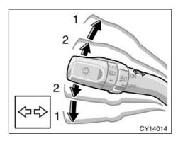
If the turn signal indicator lights (green lights) on the instrument panel flash faster than normal, a front or rear turn signal bulb is burned out.
