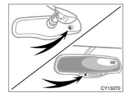
To ensure correct functioning of antiglare mirror sensors located on both sides of the mirror, do not touch or cover the sensors with your finger or a piece of cloth, etc.
