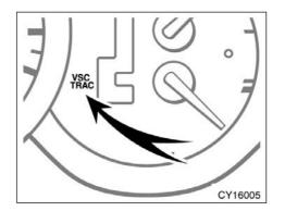
If there is any abnormality in the system, the "VSC TRAC" warning light will come on. When the "DAC" switch is pushed, the downhill assist control system indicator light also flash.
