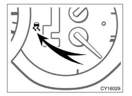
With the vehicle traveling at a speed of 25 km/h (15 mph) or less, release your foot from the accelerator or brake pedal to activate the system. The vehicle will descend the hill at a low speed. While the system is operating, the slip indicator light on the instrument panel will flash and the stop lights and high mounted stoplight will be lit.
