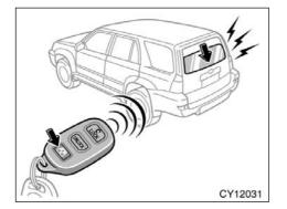
To open the back window, push the back window open switch of the transmitter for about 1 second. The window will fully open.
