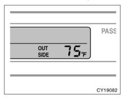
The displayed temperature ranges from  $-30^{\circ}C$  ( $-22^{\circ}F$ ) up to  $50^{\circ}C$  ( $122^{\circ}F$ ).
