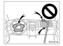
• Do not put anything or any part of your body on or in front of the dashboard or steering wheel pad that houses the front airbag system. They might restrict inflation or cause death or serious injury as they are projected rearward by the force of the deploying airbags. Likewise, the driver and front passenger should not hold objects in their arms or on their knees.
