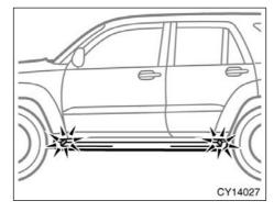
Lighting the running boards and the ground helps you easily to get in and out of the vehicle in the night. The lights come on when any of the side doors is opened.
