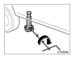
Never get under the vehicle when the vehicle is supported by the jack alone.
