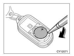
2. Remove the discharged transmitter battery by ballpoint pen.
