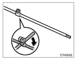
When connecting the jack handle extensions, use the jack handle to tighten the square head bolt. Make sure that the bolt fits into the depression on the joint.
