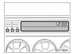
To reset the hour: Push the "H" button. To reset the minutes: Push the "M" button.
