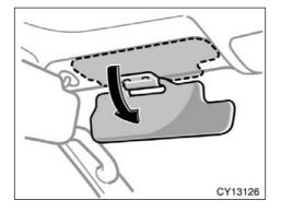
To block the glare from the front when the main sun visor is swung to the lateral side, swing down the sub visor.
