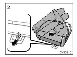
2. Unlock the seat leg by pulling the handle behind the seat, and lift the whole seat up. Retract the seat leg into the back of the seat cushion. Then, place the seat on the floor.
