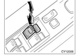
Automatic operation: Push the switch completely down or pull it completely up, and then release it. The window will fully open or close. To stop the window partway, lightly move the switch in the opposite direction and then release it.
