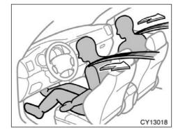
The driver and front passenger seat belt pretensioners are designed to be activated in response to a severe frontal impact. On vehicles equipped with curtain shield airbags, the pretensioners are also activated during vehicle rollover.
