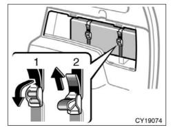
The right side of luggage compartment auxiliary box is equipped with a belt to hold the objects.
