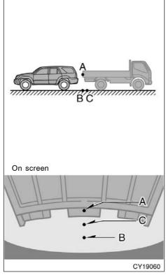
The distance that appears on the screen between three-dimensional objects (such as vehicles) and flat surfaces (such as the road) and the actual distance differ as follows.
