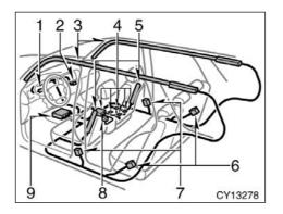
The SRS side airbag and curtain shield airbag system consists mainly of the following components, and their locations are shown in the illustration.
