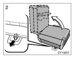
2. Unlock the seat leg by pulling the handle behind the seat, and swing the whole seat up and sideward.
