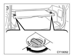
3. Turn the left and right knobs from the "UNLOCK" position to the "LOCK" position.
