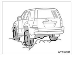
The "AUTO LSD" system aids traction by using the traction control system to control engine performance and braking when one of the rear wheels begins to spin.
