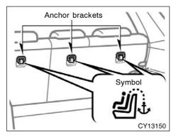
Use the anchor brackets behind the rear seatbacks to attach the top strap.
