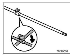
When connecting the jack handle extension(s) and jack handle end, use the jack handle to tighten the square head bolt. Make sure that the bolt fits into the depression on the joint.
