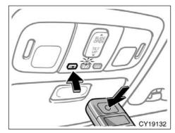
Simultaneously press and hold the hand-held garage transmitter button along with the selected HomeLink<sup>®</sup> button.
