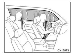
The SRS (Supplemental Restraint System) side airbags and curtain shield airbags are designed to provide further protection for the driver, front passenger and rear seat passengers<sup>\*1</sup>/second seat passengers<sup>\*2</sup> in addition to the primary safety protection provided by the seat belts.
