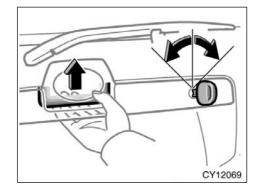
To open the back door, push up the back door opener.
