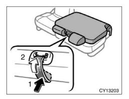
If you cannot raise the seatback because of the locked seat belt, do not try to force it. Release the lock of the seat belt in the following way.
