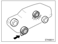
2. Block the wheel diagonally opposite the flat tire to keep the vehicle from rolling when it is jacked up.
