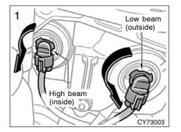
1. Turn the bulb base counterclockwise to the front of the vehicle as shown.
