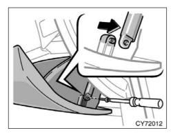
1. Open the glove box. Remove the screw with a Phillips-head screwdriver and slide the hook as shown.
