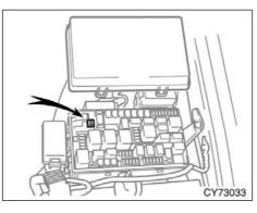
If the headlights or other electrical components do not work, check the fuses. If any of the fuses are blown, they must be replaced.
