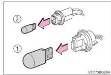
5 When installing the light bulb, install by conducting 3 and 4 with the directions reversed.
