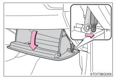
Push in each side of the glove box to disconnect the claws, and then slowly and fully open the glove box while supporting it.
