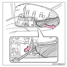
5 Remove the socket from the side turn signal light housing.
