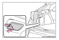
2 Pull the lever backward and check that the fuel filler door opens.
