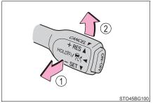
2 Pushing the lever up resumes the cruise control and returns vehicle speed to the set speed.
