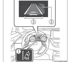
Indicates that steering wheel assistance of the steering control function is operating.
