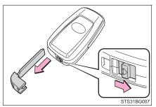
After using the mechanical key, store it in the electronic key. Carry the mechanical key together with the electronic key. If the electronic key battery is depleted or the entry function does not operate properly, you will need the mechanical key.  $(\rightarrow P. 436)$
