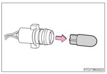
7 Replace the bulb and install the socket to the side turn signal light housing.
