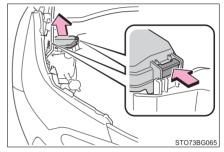
Engine compartment type B fuse box
