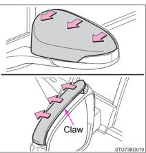
Release the claw of the bottom part of the cover and then remove the cover.
