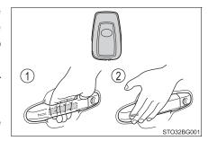
2 Touch the lock sensor (the indentation on the side of the front door handle) to lock all the doors.
