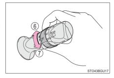
Washer/wiper dual operation Wipers will automatically operate a couple of times after the washer squirts.
