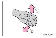
Large adjustment: Hold the lever up or down to change the speed, and release when the desired speed is reached.
