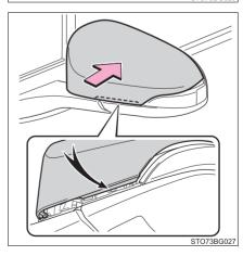
11 Attach the cover claws spanning over the entire perimeter.
