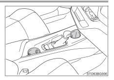
The depth of the rear side cup holder can be changed as shown in the illustration.
