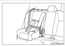
5 Fully extend the shoulder belt and allow it to retract to put it in lock mode. In lock mode, the belt cannot be extended.
