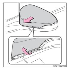
Insert a flathead screwdriver and remove the lens to the outside.
