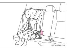
Check that the shoulder belt is correctly positioned over the child's shoulder and that the lap belt is as low as possible.  $(\rightarrow P. 26)$
