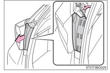
2 Remove the 2 screws and pull the light unit toward the rear of the vehicle to remove it
