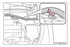
2 Disconnect the claws and remove the service cover.
