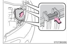
▶ Engine compartment type C fuse box
