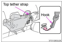
If the head restraint does not interfere with the child restraint system installation, install the head restraint.
