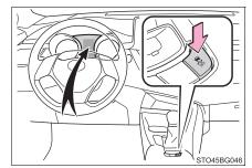
To turn the TRAC and VSC systems off, press and hold for more than 3 seconds while the vehicle is stopped.
