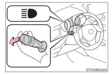
2 Press the Automatic High Beam switch.
