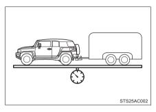
The maximum allowable gross combination weight. The gross combination weight is the sum of the total vehicle weight (including the occupants, cargo and any optional equipment installed on the vehicle) and the weight of the trailer being towed (including the cargo in the trailer).
