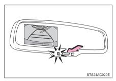
When the screen is displayed, press AUTO on the inside rear view mirror to switch the screen ON/OFF mode.
