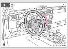
Adjust to the ideal position by moving the steering wheel vertically.
