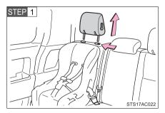
Secure the child restraint using the LATCH anchors or seat belt, and remove the head restraint.
