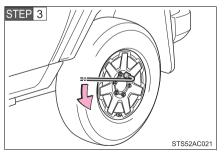
Slightly loosen the wheel nuts (one turn).
