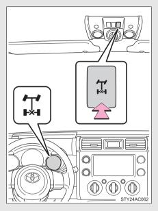
Press the RR DIFF LOCK switch to lock the rear differential.
