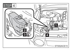
The coolant level is satisfactory if it is between the F (Full) and L (Low) lines on the reservoir.
