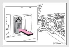
Press the CLUTCH START CANCEL switch to cancel the clutch start system with the engine switch is turned to the ON position.
