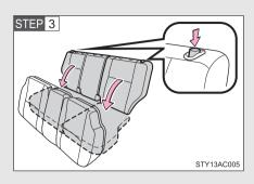
Push the lock release button and fold down the seatback.
