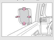
Adjust the mirror up, down, in or out by pushing the mirror surface.
