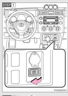
Open the cover and connect the portable audio device.
