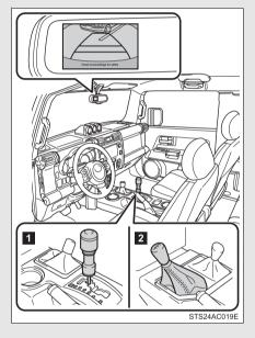
The rear view image is displayed when the shift position is in R and the engine switch is in the ON position.
