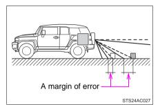
When any part of the vehicle sags due to the number of passengers or the distribution of the load, there is a margin of error between the guide lines on the screen and the actual distance/course on the road.
