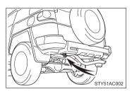
When your vehicle becomes stuck and cannot move, the emergency hook is used for another vehicle to pull your vehicle out in an emergency.
