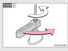
Loosen the antenna with the wrench and remove it.
