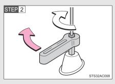
Using the wrench, tighten the antenna an additional 1/8th turn (20 to 45 degrees) to secure it in place.
