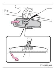
Hold and rotate the mirror to adjust the support.
