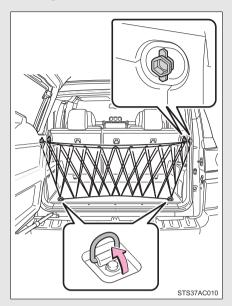
To hang the cargo net, use the cargo net hooks and tie-down hooks.
