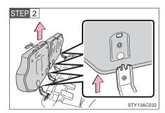
Separate the bottom cushion from the hinge.
