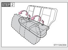
Swing the bottom cushion up by pulling the lock release strap.
