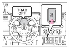
Quickly press and release the switch to turn off TRAC.
