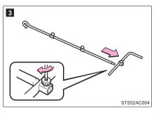
3 Assemble the jack handle extension bar and the jack handle and tighten the screw.
