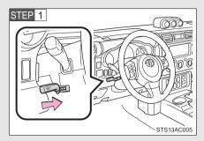
Hold the steering wheel and pull and hold the lever.
