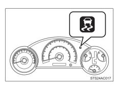
If any of the drive wheels spins, the slip indicator flashes to indicate that the active traction control system have been engaged.
