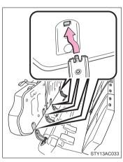
Click the claw of the hinge into the hole of the bottom cushion before refastening the dial.
