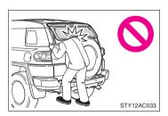
The glass hatch may suddenly shut if it is not opened fully. It is more difficult to open or close the glass hatch on an incline than on a level surface, so beware of the glass hatch unexpectedly opening or closing by itself. Make sure that the glass hatch is fully open and secure before using the luggage compartment.
