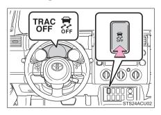
Press and hold the switch for more than 3 seconds while the vehicle is stopped to turn off TRAC and VSC.
