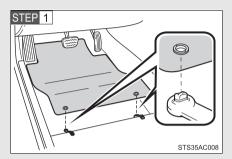
Insert the retaining hooks (clips) into the floor mat eyelets.
