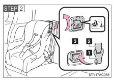
Raise the anchor bracket, latch the hook onto the anchor bracket and tighten the top tether strap.
