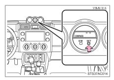
Press the SET button until the zone number appears on the outside temperature display.
