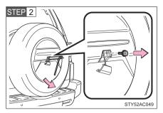
Remove the bolt which fixes the spare wheel cover using the wrench in the tool bag  $(\rightarrow P. 484)$ .
