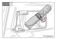
Remove the cover and loosen the strap.
