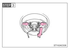
Release the bulb retaining spring.
