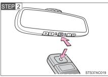
Press and hold down one of the buttons on the HomeLink<sup>®</sup> and the button on the transmitter. When the indicator on the HomeLink<sup>®</sup> changes from a slow to a rapid flash, you can release both buttons.
