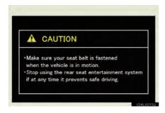
This screen appears for a few seconds when the "ENGINE START STOP" switch is in ACCESSORY or IGNITION ON mode.
