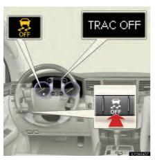
Push and hold the button for more than 3 seconds while the vehicle is stopped to turn off Active TRAC, VSC and Trailer Sway Control
