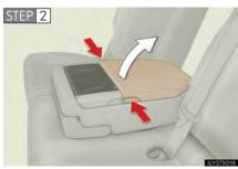
Press the button to release the lock.
