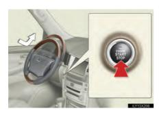
When the "ENGINE START STOP" switch is turned OFF and the driver's seat belt is unfastened, the steering wheel returns to its stowed position by moving up and away to enable easier driver entry and exit.
