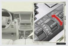
Operate the Multi-terrain Select mode select switch during Multi-terrain Select control to select a mode.
