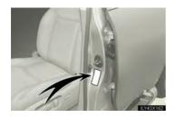
For the GAWR, see the Certification Label. For the maximum load of the tire, see the load limit at maximum cold tire inflation pressure mentioned on the sidewall of the tire.  $(\rightarrow P. 895)$
