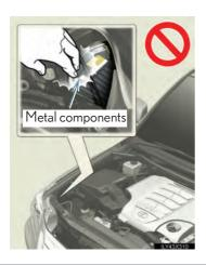
While the low beam headlights are turned on, and for a short time after they have been turned off, metal components at the rear of the headlight assembly will be extremely hot.
