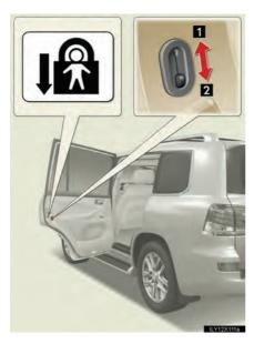
The door cannot be opened from inside the vehicle when the locks are set.
