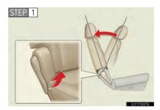
Fold the seatback while pulling the seatback angle lever. Return the seatback and secure it at the first lock position.
