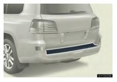
The rear step bumper is for rear end protection and easier step-up loading.
