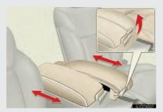
Lift the lid while pulling up the upper lever to release the lock.
