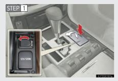
Press the lid, open the cover and connect the portable audio device.
