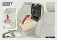
Lift the lid while pulling up the lower lever to release the lock.
