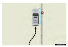
Use the vehicle width line to check the vehicle's distance from objects such as curbstones etc. As shown in the illustration, be sure that the vehicle width line does not overlap the object. If you also move the vehicle so that the vehicle width line and the object are parallel, you can park parallel to the object
