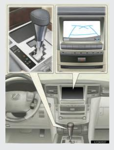
The parking assist monitor system will activate when the shift lever is in "R".
