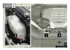
The coolant level is satisfactory if it is between the "F" and "L" lines on the reservoir.
