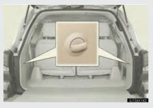
To hang the cargo net, use the cargo net hooks and rear cargo hooks.
