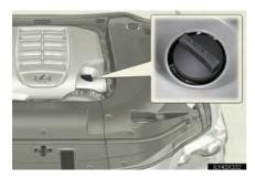
If the oil level is below or near the low level mark, add engine oil of the same type as already in the engine.  $(\rightarrow P. 883)$
