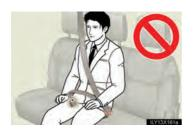
Do not use the third center seat belt with either buckle released. Fastening only one of the buckles may result in death or serious injury in case of sudden braking, sudden swerving or an accident.
