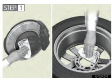
Remove any dirt or foreign matter from the wheel contact surface.
