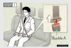
Push the release button on buckle A
