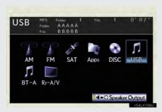
Select USB mode on the source screen to display the control screen.
