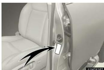
For the GAWR, see the Certification Label. For the maximum load of the tire, see the load limit at maximum cold tire inflation pressure mentioned on the sidewall of the tire. (→P. 697)
