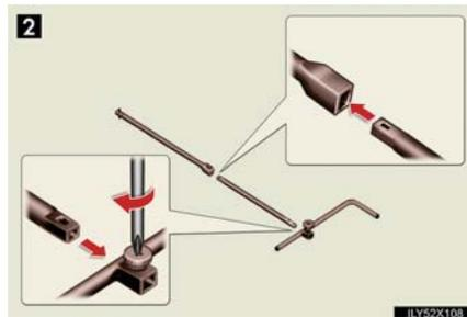
**2** Assemble the jack handle and the jack handle extension bar and tighten the screw.
