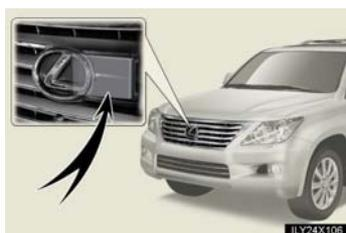
Always keep the sensor and grille cover clean to ensure that the vehicle-to-vehicle distance control operates properly. (Some obstructions, such as snow, ice or plastic objects, cannot be detected by the obstruction sensor.)
