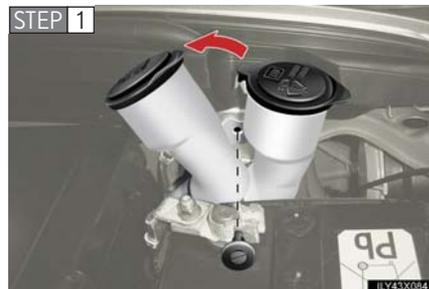
For the left side only: Remove the securing bolt and move the washer fluid filler opener.
