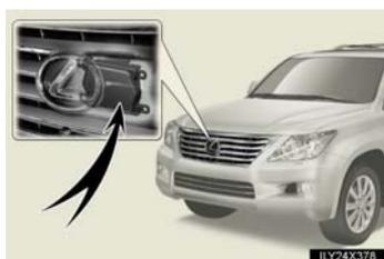
If the dynamic radar cruise control is used on a road with very light traffic and very little to reflect the radar waves emitted by the radar sensor, the system may decide that the radar sensor is dirty, even if the sensor is not actually dirty. In this case, switch to the conventional constant speed control mode. (→P. 209)
