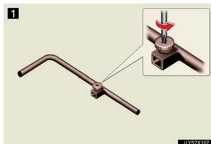
**1** Loosen the screw using a screwdriver.
