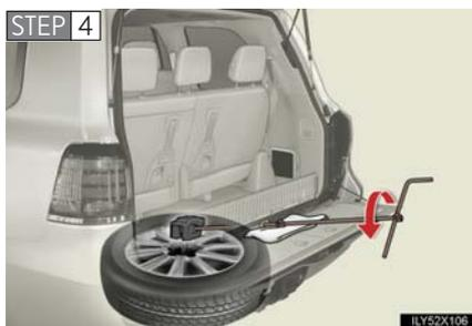
Lower the spare tire completely to the ground.
