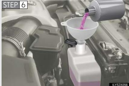
Add engine coolant if necessary.
