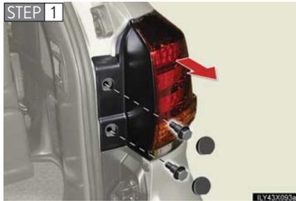
Open the back door and remove the bolts and lamp assembly.
