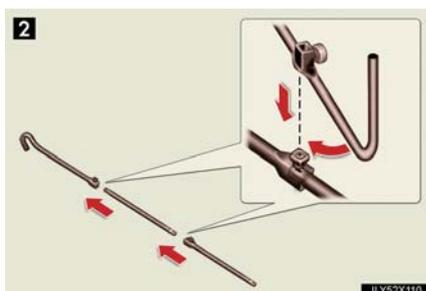
2 Assemble the jack handle extension bar and the jack handle bar and tighten the bolts.
