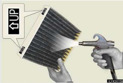
If the filter is dirty, clean by blowing compressed air through the filter from the downward side.
