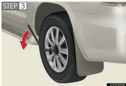
Slightly loosen the wheel nuts (one turn).
