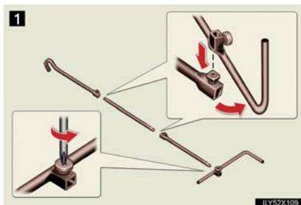
1 Loosen the bolts and the screw using either the jack handle or a screwdriver.
