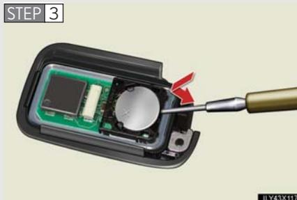
Remove the depleted battery.
