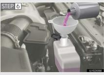
Add engine coolant if necessary.
