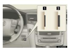
Turn the main switch to disable the power back door system.
