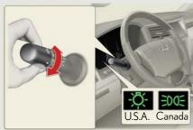
The side marker, parking, tail, license plate, daytime running lights and instrument panel lights turn on.
