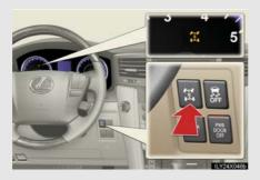
Lock the center differential when your vehicle's wheels get stuck in a ditch or when driving on a slippery or bumpy surface.
