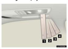
The display angles change as follows each time "TILT" is pressed.
