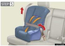
While pushing the child restraint system into the second seat, allow the shoulder belt to retract until the child restraint system is securely in place.
