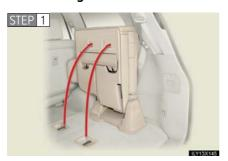
Remove the seat hook covers from the floor and install them into the underside of the seat cushion.
