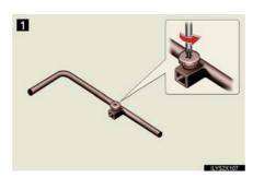
**1** Loosen the screw using a screwdriver.
