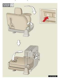
If the switch is pressed, the seat will automatically fold and lift sideward.
