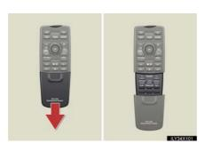
To use the buttons under the cover, slide the cover down.
