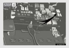
Remove the fuse with the pull-out tool.
