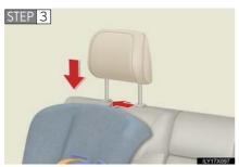
Outside only: Adjust the head restraint to the downmost position.
