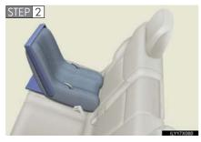
Place the child restraint system on the second seat facing the rear of the vehicle.
