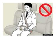
Do not use the third center seat belt with either buckle released. Fastening only one of the buckles may result in death or serious injury in case of sudden braking, sudden swerving or a collision.
