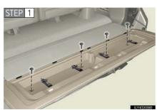
Open the back door and remove the bolts and the cover.
