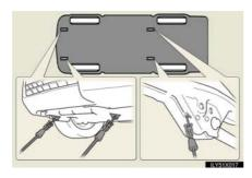
If your Lexus is transported by a flat bed truck, it should be tied down at the locations shown in the illustration. When attaching the hooks to the rear of the vehicle, make sure to attach them to the inside of the vehicle.
