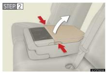
Press the button to release the lock.
