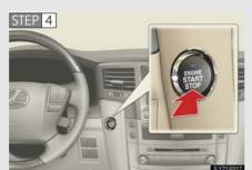
Press the "ENGINE START STOP" switch.
