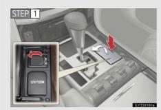
Connect the portable audio device.
