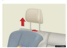
Adjust the head restraint to the upmost position.
