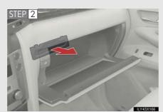
Open the glove box and remove the filter cover.
