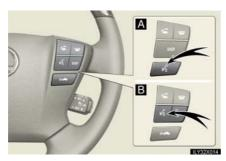
Press or to operate the voice command system. (\( \rightarrow "Navigation System Owner's Manual")
