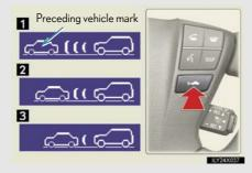
Each press of the switch changes the vehicle-to-vehicle distance.
