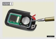
Remove the depleted battery.
