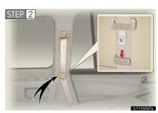
Pass the outer seat belts through the seat belt hangers and secure the seat belt plates.
