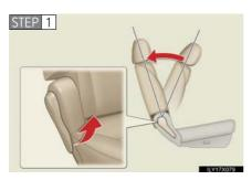
Fold the seatback while pulling the seatback angle lever. Return the seatback and secure it at the first lock position.
