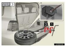
Insert the jack handle extension into the lowering screw.
