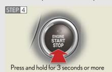
Stop the engine by pressing and holding the "ENGINE START STOP" switch for 3 consecutive seconds or more.
