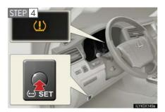
Push and hold the tire pressure warning reset switch until the tire pressure warning light blinks slowly 3 times and a message appears on the multi-information display.
