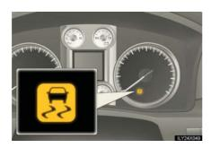
If the vehicle is in danger of slipping, rolling backwards when starting on an incline, or if the wheels spin, the slip indicator light flashes to indicate that the VSC/Active TRAC/hill-start assist control systems have been engaged.
