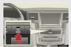
The operation time changes according to the ambient temperature and vehicle speed. Pressing the button again also turns the defoggers off.
