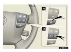
Press or to operate the voice command system. (\(\rightarrow\)"Navigation System Owner's Manual")
