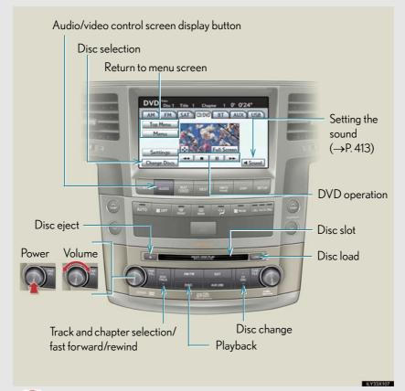
If  $\bigcirc$  appears on the screen when you touch an icon, the operation relevant to that control is not permitted.
