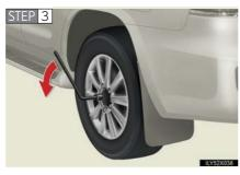
Slightly loosen the wheel nuts (one turn).
