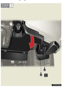
Remove the fender liner bolts, loose the fender liner nut and remove the fender liner.
