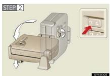
If the switch is held down the seat will automatically return to the folding position. (Buzzer sounds twice)
