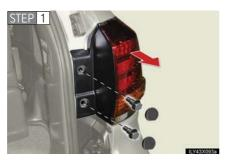
Open the back door and remove the bolts and lamp assembly.
