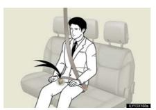
Make sure that the buckle with the gray buckle release button is securely latched for ready use of the center seat belt.
