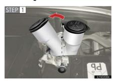
For the left side only: Remove the securing bolt and move the washer fluid filler opener.
