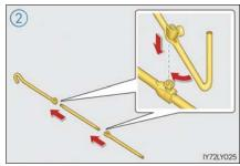
Check that the screw is firmly tightened.
