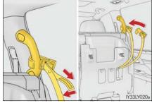
3 Remove the seat hook covers from the back of the seat cushion, and install them on the seat hooks.
