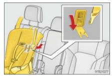
3 Adjust the head restraint to the downmost position.
