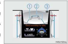
Indicates that the under vehicle terrain view display is of an image taken in the past.
