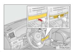
2 Press the power supply switch of the wireless charger.
