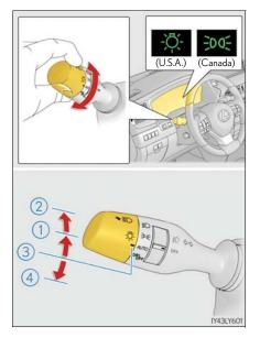
1 With the headlights on, push the lever forward to turn on the high beams.
