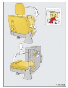
Remove the seat hook covers from the underside of the seat cushion, and install them on the seat hooks.
