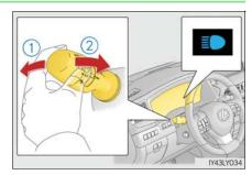
2 Pull the lever toward you to turn on the high beams.
