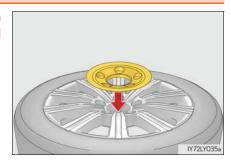
2 Install the holding bracket, inserting the claw into the wheel lug nut hole. Turn the jack handle extension clockwise to take up slack in the chain.
