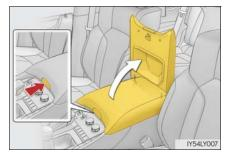
2 Turns the cool box on/off When on, the indicator light comes on.
