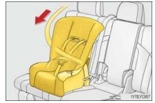
S While pushing the child restraint system into the second seat, allow the shoulder belt to retract until the child restraint system is securely in place.
