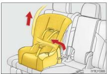
6 If the child restraint system has a top tether strap, the top tether strap should be latched onto the top tether strap anchor. (→P. 69)
