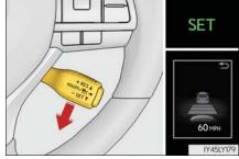
If the lever is operated while the vehicle speed is below approximately 30 mph (50 km/h) and a preceding vehicle is present, the set speed will be adjusted to approximately 30 mph (50 km/h).
