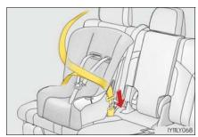
4 Fully extend the shoulder strap and then allow it to retract slightly into the ALR lock mode.
