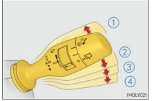
The sensor sensitivity can be adjusted when "AUTO" is selected.
