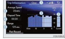
Average fuel consumption for the past 15 minutes is divided by color into past averages and averages attained since the engine switch was last turned to IGNITION ON mode. Use the displayed average fuel consumption as a reference.
