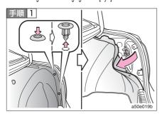
It opens a trunk, the clip (2 pieces) is removed, and the cover is turned over.
