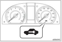
The security pilot light in the meter blinks to inform them of the operation of the system when "Engine start stop" switch is turned off.
