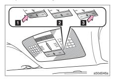
It synchronizes when the switch is operated and the [riya] reading light operates.
