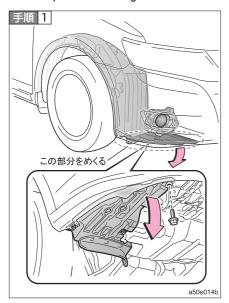
The screw (1) is detached, and the fender liner is turned over.
