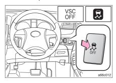
The switch is pushed to stop TRC and VSC when stopping, and it maintains it for about three seconds or more.
