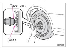
seat of the wheel when substituting it from the aluminum foil to the temporal spare tire.
