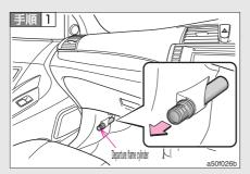
The departure flame cylinder of one's passenger's seat feet is taken out.
