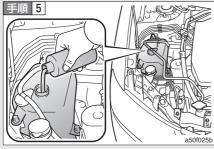
When cooling water is insufficient, cooling water is replenished (P. 296).
