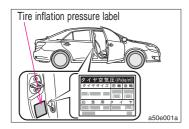
The air pressure in the tires can be confirmed with the tire inflation pressure label on the driver side.
