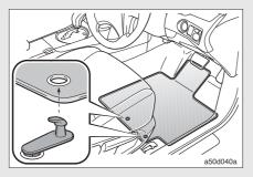
In the carpet, there is a hole for the fixed clip installation of the floor mat.
