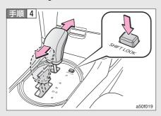
The shift lock release button is pushed.
