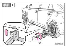
Part A of the jack is spent by the hand, and the jack ditch is put on the jack set position firmly.
