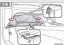
An upper tab is detached pushing the glove box side internally, and one side removes and detaches a feretory and lower tab.
