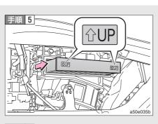
The filter is detached, and it exchanges it for a new filter.
