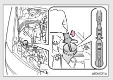
Please replenish the washer fluid when the liquid level approaches the position of LOW.
