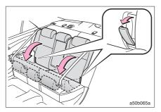
The back also knocks down the drip forward while pulling a lever.
