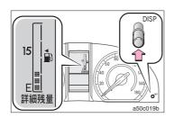
When confirming it, the DISP button (Or, DISP switch \*) is pushed while displayed for the distance that can cruise on the multi information display.
