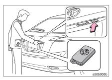
The trunk opening switch is unlocked pushing.
