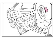
The [riya] seat door doesn't open from the inside when making it to the lock side.
