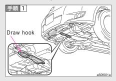
The draw hook is roped so that the wound should not place to the body.
