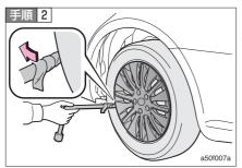
The hubcap is removed (Only the steel wheel :).
