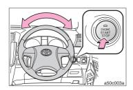
Please push "Engine start stop" switch while moving the steering wheel right and left.
