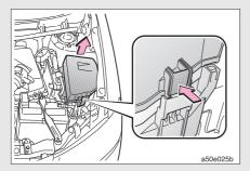
The cover is lifted while pushing the tab.
