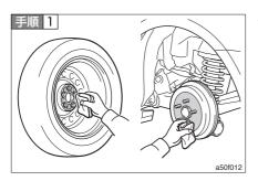
The dirt of the wheel contact side is wiped off.
