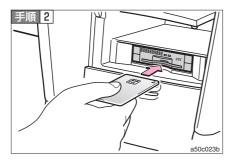
The cap of central box ( P. 200) is opened, and the ETC card is inserted.
