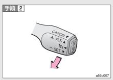
It acceleration/decelerates up to the speed of hope, and the lever is lowered.
