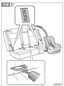
The position of the bar only for fixation is confirmed, and the child seat is installed in the seat.
