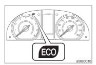
It is informed that the ecodrive with a little amount of CO2 (carbon dioxide) exhaust is done them when the ecodrive indicator lights. It turns it off when stepping on the gas pedal more than the necessity. (Operate at D position.)
