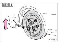
The nut is firmly tightened 2 and three times by the numerical order of figure.
