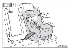
It is confirmed to shake the installed child seat lightly, and to be fixed surely.
