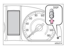
To switch the display, the DISP button is pushed.
