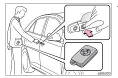
The lock switch is locked pushing.
