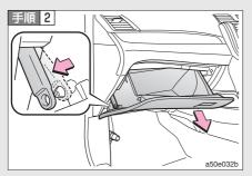
removed and the pin of opening [danpa-sute-] is removed.
