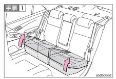
The region of the lateral zone of the seat cushion in the forward end is lifted, and the lock is released.
