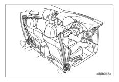
It contributes to securing an appropriate effect of the crew restraint by drawing in the seat belt when a strong collision is received forward.
