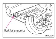
The one used when dragging it to another car in the emergency when it becomes impossible to run by stacking because of the snowdrift etc. Another car cannot be pulled.
