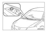
Please paste to the window glass neither putting the thing on the sensor nor closing the sensor. Neither an automatic lighting nor the turning off function work normally when light from surroundings is shut out.
