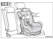
It is confirmed to shake the installed child seat lightly, and to be fixed surely.
