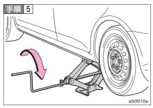
The body is raised from ground to a little parting of the tire.
