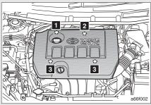
Each part of the cover is pulled up in the following order, and the cover is removed from a fixed pin on the entine side.
