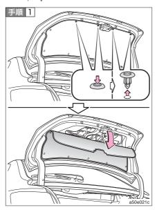
It opens a trunk, the clip (4 pieces) is removed, and the cover is turned over.
