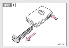
A mechanical key is pulled out.
