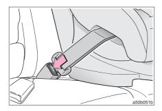
When it unbuckles and it winds up up the belt fully, the child seat fixation mechanism is released.
