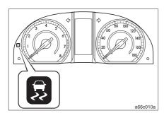
The slipping pilot light blinks to display the operation of VSC and TRC when the vehicle seems to sideslip, becomes, and the drive wheel runs idle.
