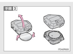
The module cover is removed by using the coin etc., and the consumed battery is taken out.
