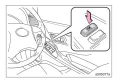
If the switch is pushed, operating the door glass other than the driver's seat becomes impossible.
