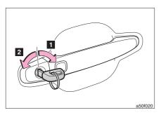
The door can be locked and be unlocked with mechanical key (P. 20).
