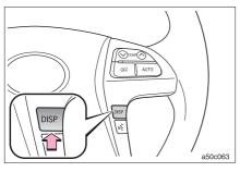
The navigation system installation car of the manufacturer option can switch the display with the DISP switch that exists in the steering wheel.
